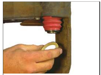
Figure 84 – Place the Retaining Ring onto the Groove in the Guide Pin
