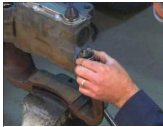
Figure 79 – Position the New Bushing
