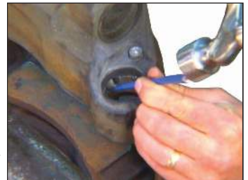
Figure 74– Remove the Tab that Holds the Bushing in Position
