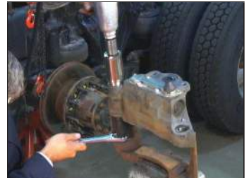
Figure 72 – Remove the Long Guide Pin
