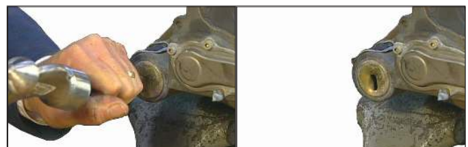
Figure 64 – Punch Guide Pin Cap (10)
