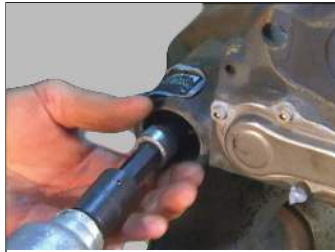
Figure 68 – Remove the Caliper Bolts
