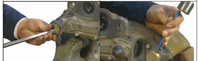
Figure 66 – Pry to Remove Guide Pin Cap (10)
