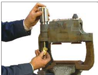
Figure 71 – Install the Removal Tool
