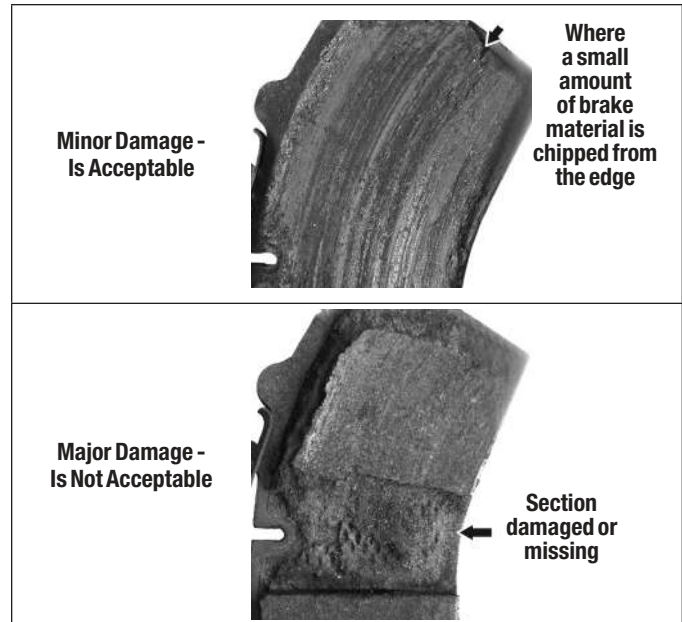
Figure 24 – Brake Pad Surface Inspection
