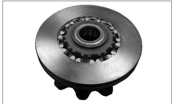
Figure 91 – Intermediate Elements (Spacers Installed)
