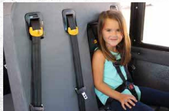
Interchangeable SafeGuard BTI seating exclusively for IC Bus® vehicles is continually compliance tested to make sure it meets and exceeds all federal safety standards
