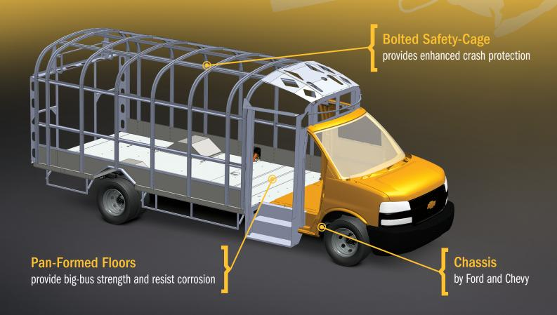
Offering a family of single and dual wheel models, **Trans Tech** buses provide big-bus strength and enhanced crash protection.
